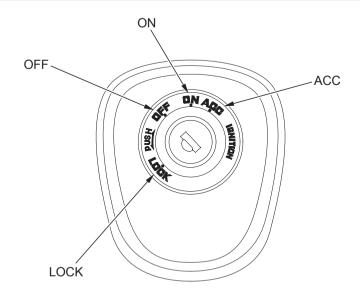
The ignition switch is used for starting and stopping the engine (page 71) and to lock the steering for theft prevention (page 87). Insert the key and turn it to the right for the ON and ACC (accessory) positions.
