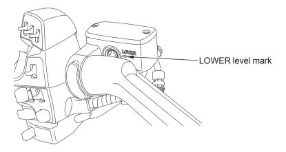
Check that the fluid level is above the LOWER level mark. If the fluid level is below the LOWER level mark, it indicates fluid leakage. See your dealer for repair.
