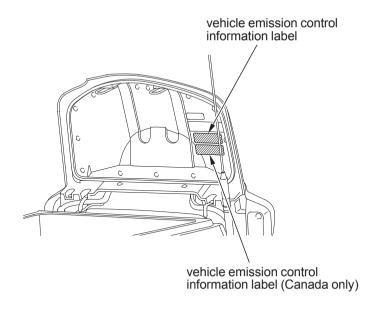
The Vehicle Emission Control Information label is attached inside the trunk lid
