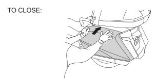
To shut each compartment, place your hands flat on the edges of its lid and press down until it is firmly closed and check the travel trunk & saddlebags open indicator is not displayed.
