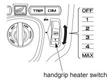
To warm up the handgrip heaters, turn the handgrip heater switch toward the MAX position.
