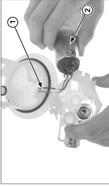
(1) CABLE TERMINALS (2) PUMP ENGINE/FILTER
