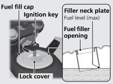
Do not fill with fuel above the plate. **Fuel type:** Unleaded gasoline only **Recommended fuel octane number:**Pump Octane Number (PON) 86 or higher. **Tank capacity:** 1.45 US gal (5.5 liters)
