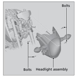
**1.** Remove the bolts and headlight assembly.
