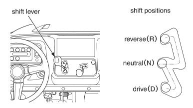
You should move the shift lever only when the vehicle is stopped with your foot on the brake pedal and with the engine idling. Use a firm motion to select the appropriate gear. Have your vehicle checked by a dealer if you experience any shifting problems.
