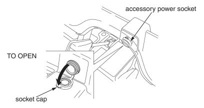
To use the accessory power socket, the engine must be on and idling.
