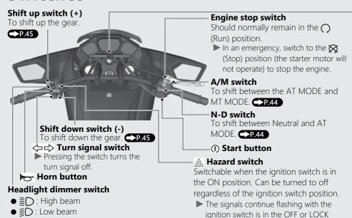
position after the hazard switch is on.
