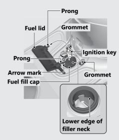
Do not fill with fuel above the lower edge of the filler neck
