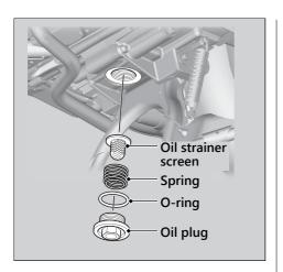
**10.** Install the oil strainer screen, spring and oil plug and tighten.
