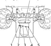
The spring pre-load adjuster has 5 positions for different load or riding conditions. Before adjusting the spring pre-load, jack up your Honda SXS (page 144) to avoid damaging the adjusters.
