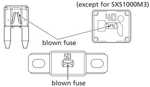
Check all the fuses before looking elsewhere for another possible cause of the problem. Replace any blown fuses and check component operation.
