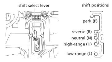
You should shift the shift select lever only when the vehicle is stopped with your foot on the brake pedal and with the engine idling. Use a firm motion to select the appropriate gear. Have your vehicle checked by a dealer if you experience any shifting problems.
