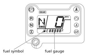
Regardless of what mode the display is in, when the fuel level reaches only one segment remaining, the display will automatically switch to the fuel gauge display. You should refuel as soon as possible.
