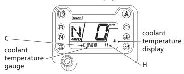
If all sections of the coolant temperature gauge, including segment H and high coolant/oil temperature indicator are on (automatically appears in the display), stop the engine and check the reserve tank coolant level.
