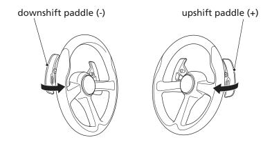
Pull the upshift paddle (+) to shift to a higher gear position and the downshift paddle (-) to shift to a lower gear position.
