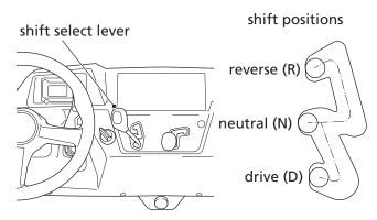
You should move the shift select lever only when the vehicle is stopped with your foot on the brake pedal and with the engine idling. Use a firm motion to select the appropriate gear. Have your vehicle checked by a dealer if you experience any shifting problems.
