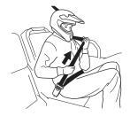
To unlatch a seat belt, press the red PUSH button on the buckles.
