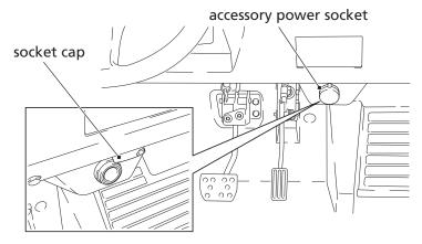
To use the accessory power socket, the engine must be on and idling.
