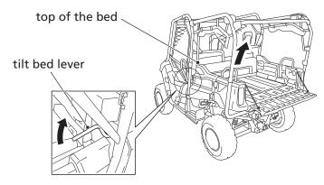
To lower the cargo bed, make sure that the area under the front of the cargo bed is clear, then manually push down on the top of the bed.
