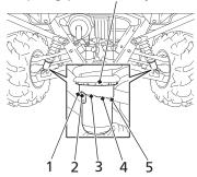
The spring pre-load adjuster has 5 positions for different load or driving conditions. Before adjusting the spring pre-load, jack up your Honda SXS (page 123) to avoid damaging the adjusters.
