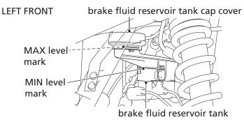
It should be between the MIN and MAX level marks. If the level is at or below the MIN level mark, check the brake pads for wear (page 170).
