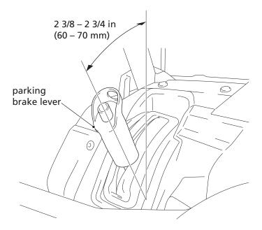
If adjustment is necessary, have the parking brake adjusted by your dealer.
