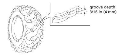
To check the condition of a tire tread, measure the groove depth in the center of the tire.
