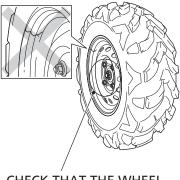
CHECK THAT THE WHEEL NUTS ARE TIGHT SXS700M2D/M4D (Aluminum wheel model)
