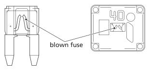
Check all the fuses before looking elsewhere for another possible cause of the problem. Replace any blown fuses and check component operation.
