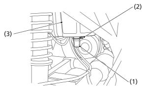
(1) drain tube(3) air cleaner housing(2) clip
