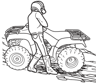
Body position for backing down a hill.
