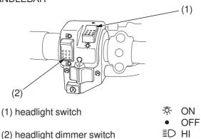
The headlight switch (1) is used to turn the headlight ON (  $\mbox{\ensuremath{\%}}$  ) or OFF (  $\mbox{\ensuremath{\bullet}}$  ). To operate, turn the switch to ON ( $\mbox{\ensuremath{\%}}$  ) or OFF ( $\mbox{\ensuremath{\bullet}}$  ).
