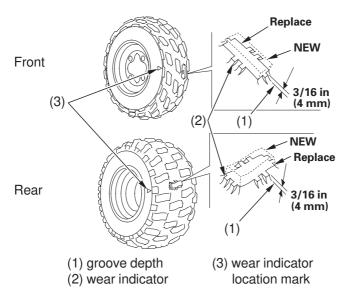
To check the condition of a tire tread, measure the groove depth (1) in the center of the tire, or check the wear indicator (2).
