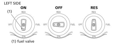
The manual fuel valve (1) is located on the left side of the fuel tank.
