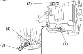
(1) oil drain plug(2) oil fill cap
