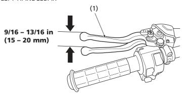
(1) rear brake lever/parking brake lever
