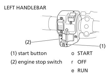
The start button (1) is used for starting the engine. Pushing the button in starts the engine. See *Starting Procedure*, page 49.
