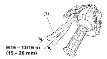
(1) rear brake lever/parking brake lever
