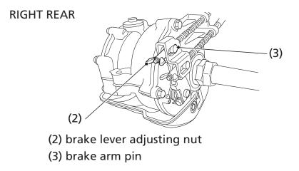
Adjust the freeplay of the rear brake lever/parking brake lever with the front wheels pointed straight ahead.
