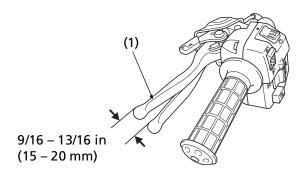
(1) rear brake lever/parking brake lever
