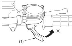
(1) throttle lever(A) to open the throttle
