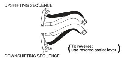
Your ATV has five forward gears (1, 2, 3, 4 and 5). To shift the transmission, pull in the clutch lever/parking brake lever, then operate the shift lever as follows.
