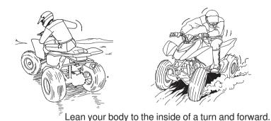
To make a turn on level ground: Steer the handlebar and lean your body toward the inside of the turn. Leaning helps balance the vehicle, and it feels more comfortable. Leaning into a turn is an important technique to master in riding an ATV.
