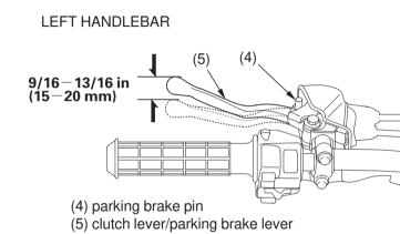
5. After parking brake adjustment is completed, adjust the clutch freeplay to the correct specification (page 106).
