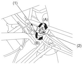
(1) brake light switch(2) adjusting nut
