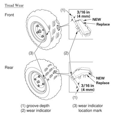
To check the condition of a tire tread, measure the groove depth (1) in the center of the tire, or check the wear indicator (2).
