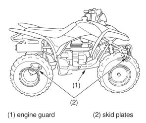
The engine guard (1) protects the engine crankcase.
