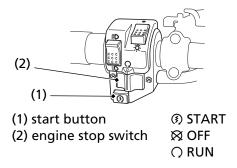
The start button (1) is used for starting the engine. Pushing the button in starts the engine. See *Starting Procedure*, page 47.
