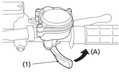
(1) throttle lever(A) to open the throttle
