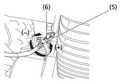
(5) lower adjusting nut(6) lower lock nut
